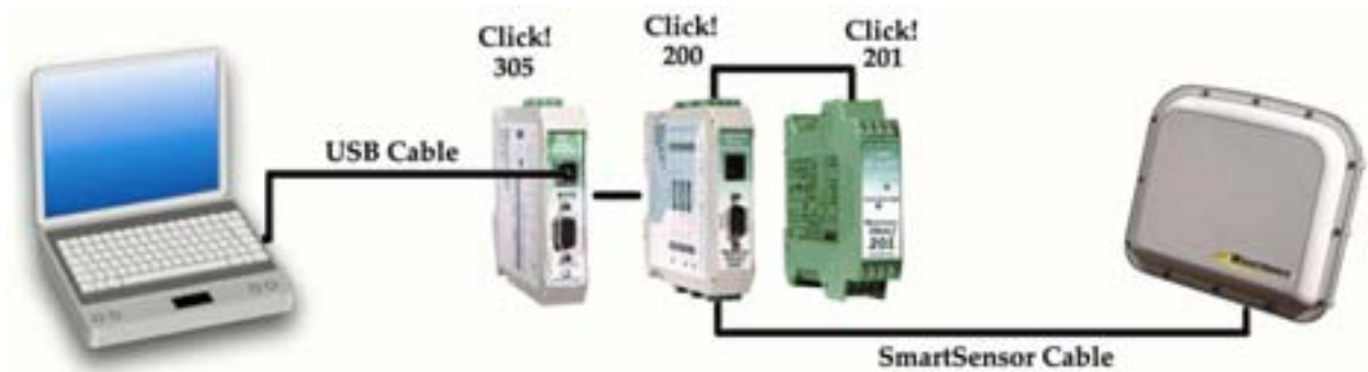
Figure 12 – USB cable connection
