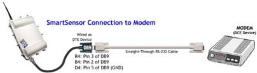
Figure 35 - Connecting a Modem to the SmartSensor
