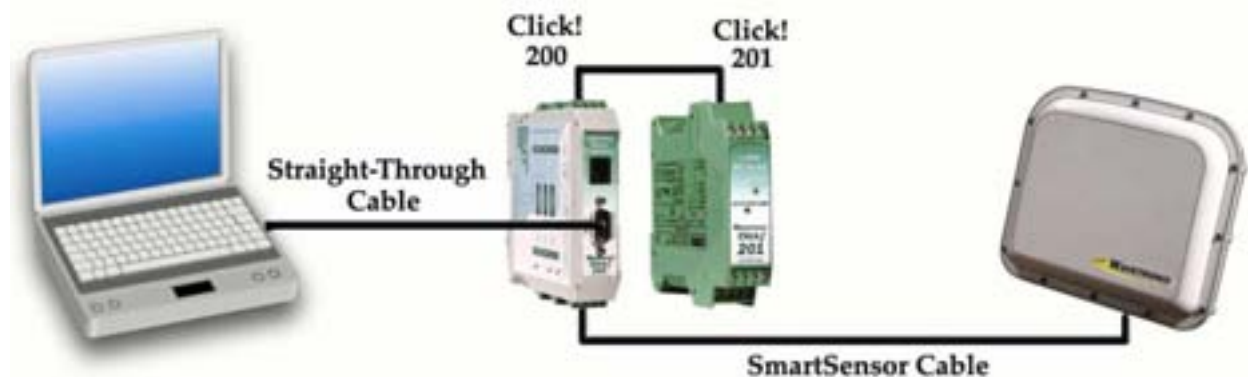
Figure 11 – Straight-through cable connection
